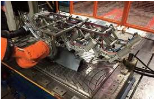
High grade SMC based material being placed in to an Aqua-floor shower deck mould using the UK's most technically advanced robotic SMC production line.
